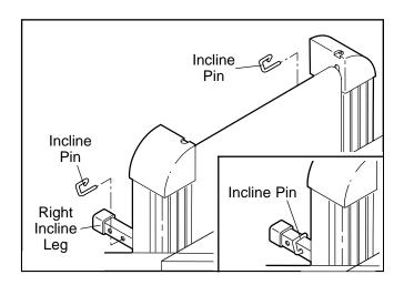
CAUTION: Before using the treadmill, make sure that both incline pins are fully inserted at the same height. Do not use the treadmill with the incline pins removed. After you have adjusted the incline legs, lower the treadmill (see HOW TO LOWER THE TREADMILL FOR USE on page 11).
